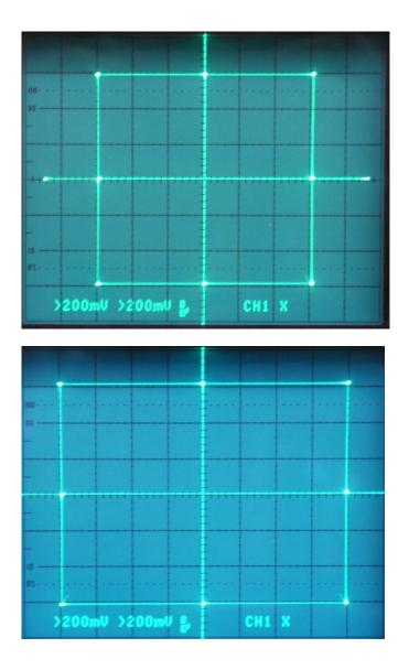
In the photo above the scope's X gain was simply set higher than the Y so the scan box becomes a rectangle.
