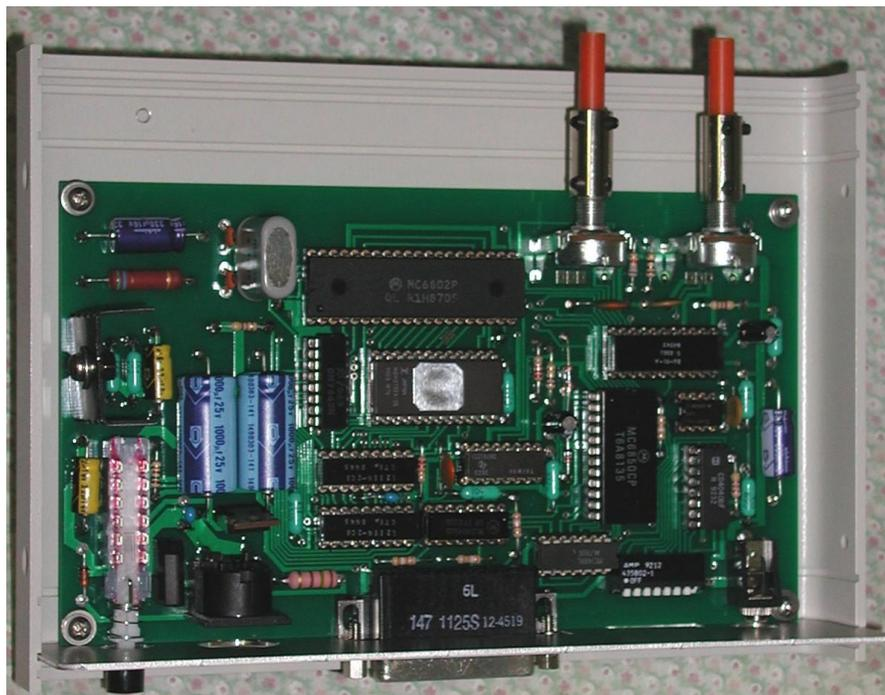
I stuck to the original style Din power connector, DIP baud rate switch, a long reach DB25 connector, the same design power switch and audio output jack. Therefore the rear panel looks near identical to Votrax's original unit:
