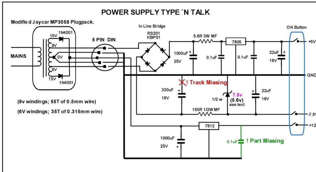
So I acquired a standard mains voltage (230V here) to 12VAC 1.67A rated Jaycar Powertech adapter, disassembled it and rewound its secondary bobbin.
