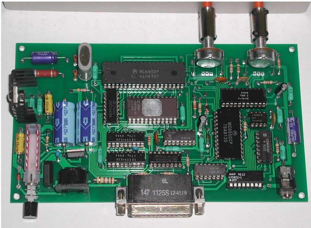
The 0.1uF ceramic bypass capacitors I used are a vintage type made by the Corning Glass Works. The originals on Votrax's pcb were blue. Mostly axial 0.1uF ceramic capacitors are a mustard-yellow color these days.
