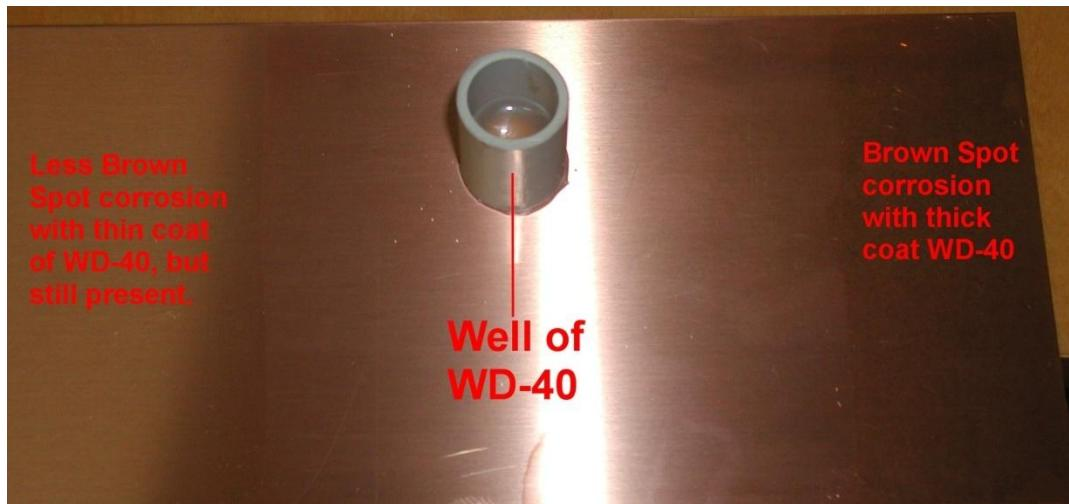
After 10 days I removed the well and inspected the copper surface in the base of the well. No corrosion at all. This confirmed that WD-40 does not actually harbour any chemical that directly attacks copper.
