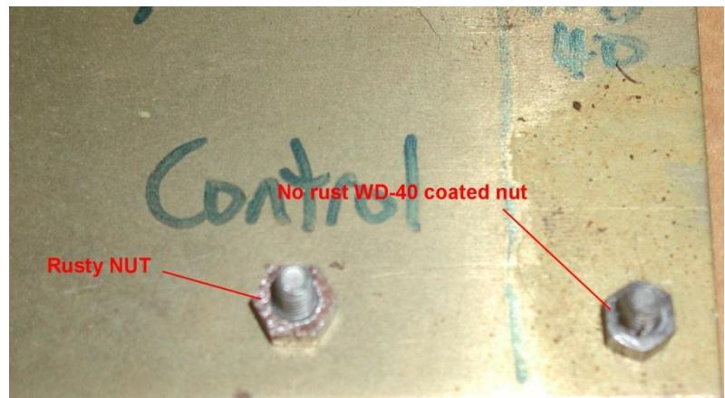
As one might have expected, the WD-40 coated nut was free from rust, but the bare one has significant surface rusting. I then removed the nuts to check for any reaction between the brass and the steel:
