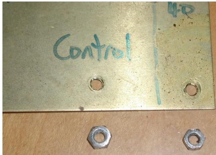
There is no visible reaction between either steel nut and the brass plate. Certainly no evidence of any green corrosion.
