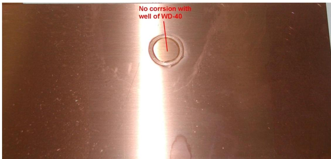
This photo shows a close up view of the WD-40 induced brown spot corrosion on copper plate:
