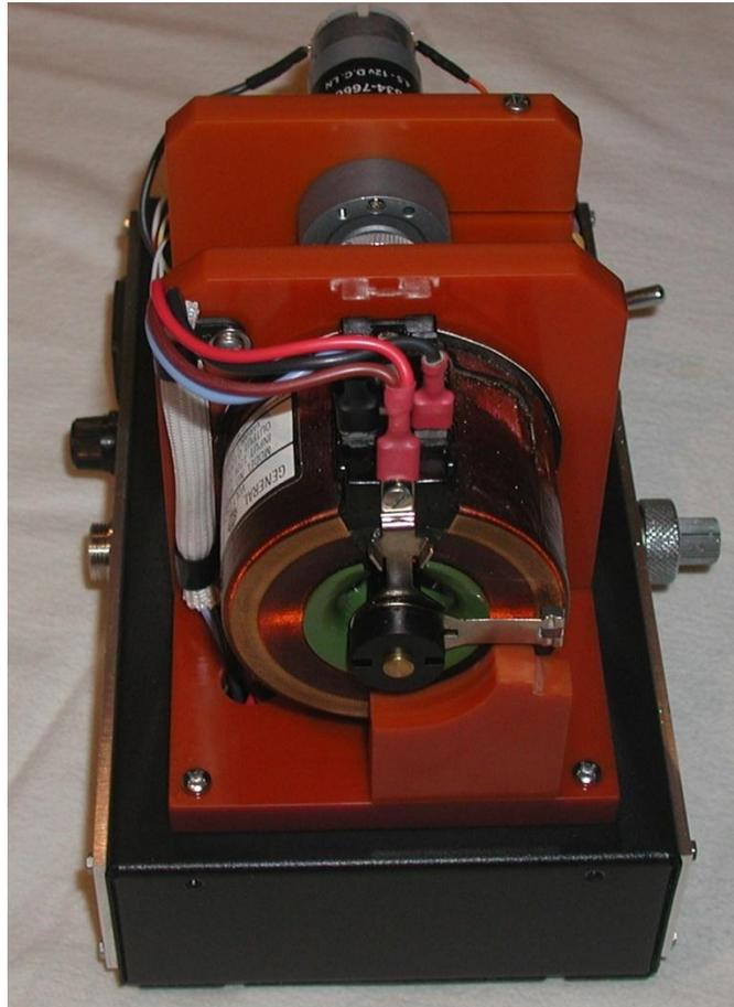
The rear view above shows the Variac's low voltage mechanical stop.
