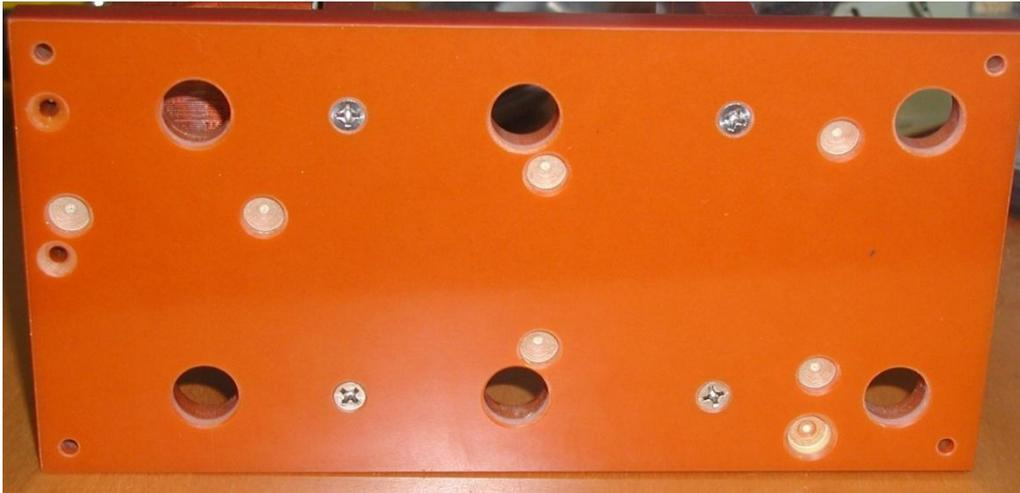
The phenolic insulating material takes a 6-32 UNC thread very well and this simplifies the construction using CS head stainless steel machine screws.
