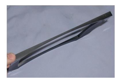
The next task was to make 8 metal bars (10mm square aluminium). This was a long process done on my small hobby lathe and drill press. There are a total of 40 holes (for
