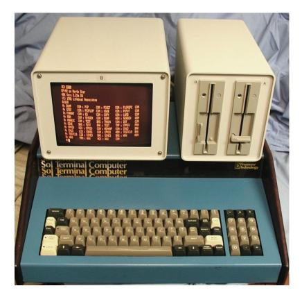
These cases are extruded aluminium and have a tough coating applied at the factory. The front and rear panels fit in grooves in the extrusion.
