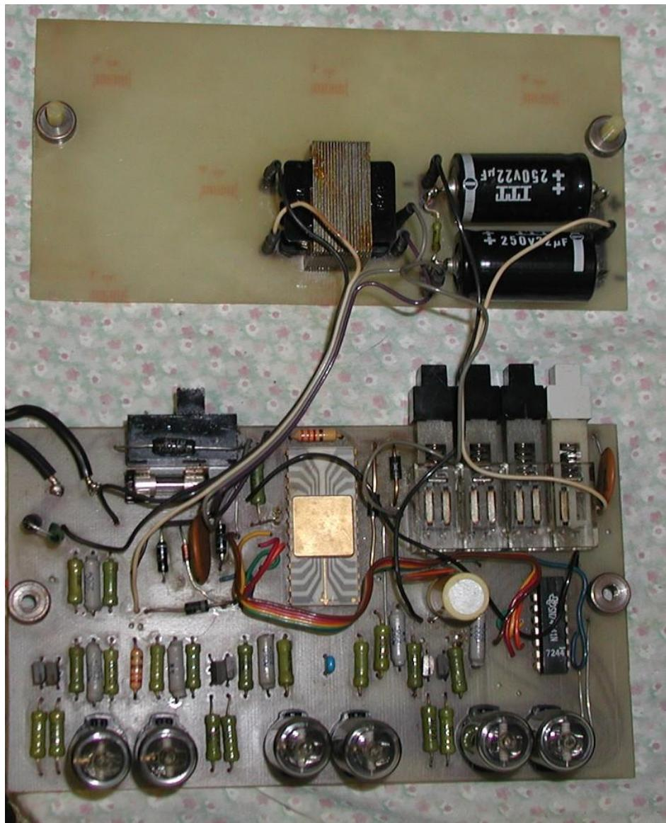
Ribbon cable connects the two pcb's and also the BCD data from the LSI chip is connected to the display driver IC (a SN74141) by a section of ribbon cable rather than pcb tracks. The green resistors are Russian made which is interesting.
