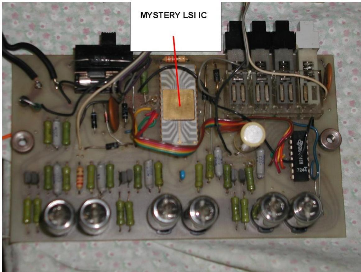
The clock had been modified by the manufacturers for the American market. There is a voltage doubler circuit for the nixie anode supply and also a two transistor circuit built on vero board.
