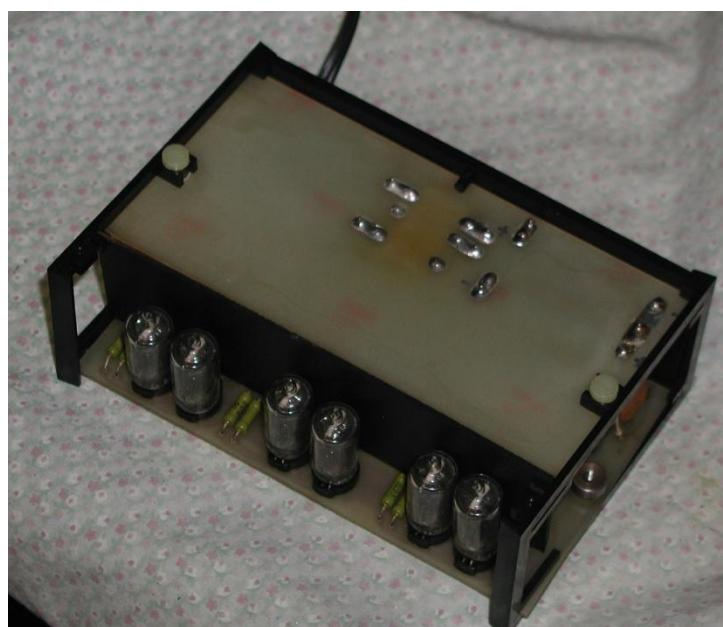
The housing is elegant, unpretentious and cleverly put together. There are two side plates, the rear and front panels and the two PCB's. When assembled as shown in the photo above they fit neatly into the external housing. The top PCB contains the power supply components. The photo below shows the two PCB's on the component surfaces:
