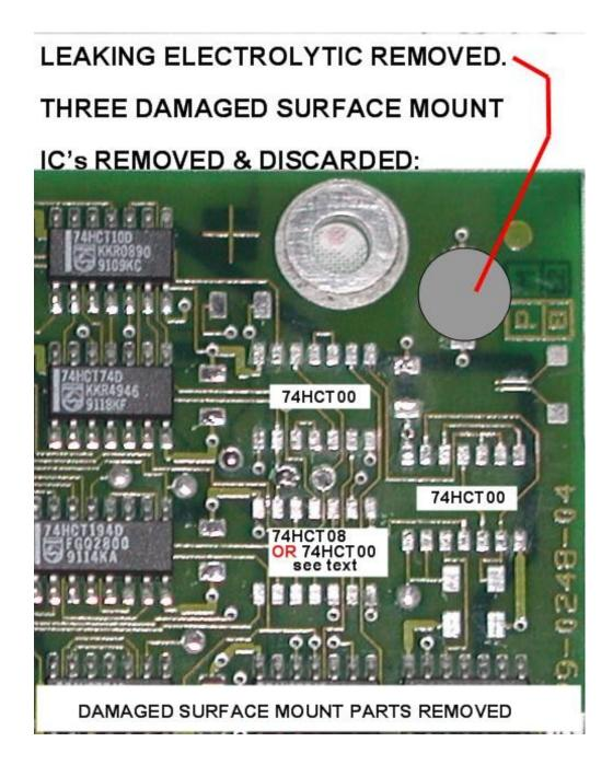
The following photos show the rebuilt pcb:
