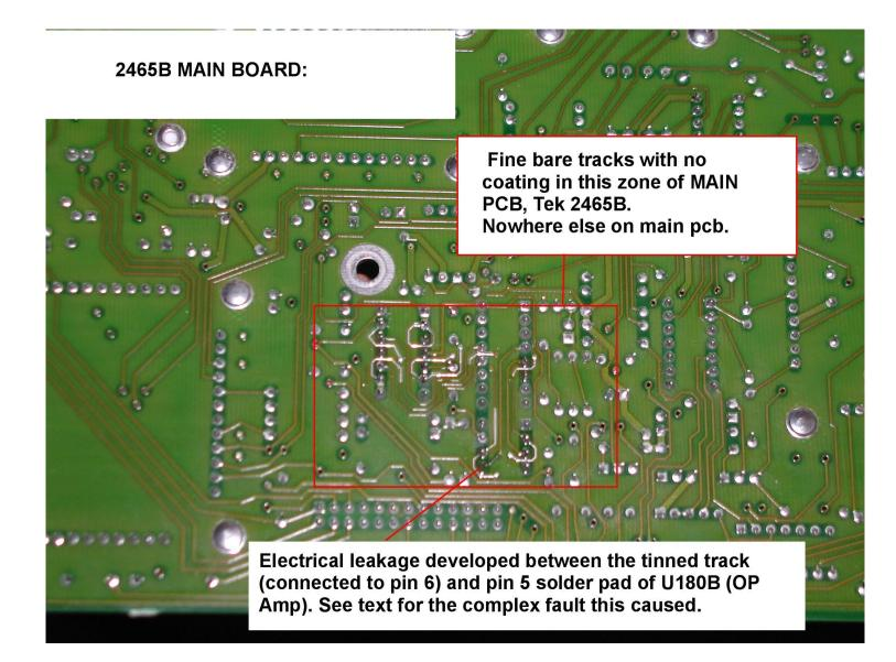
A leakage conduction pathway between pins 5 & 6 of U180B developed with time.
