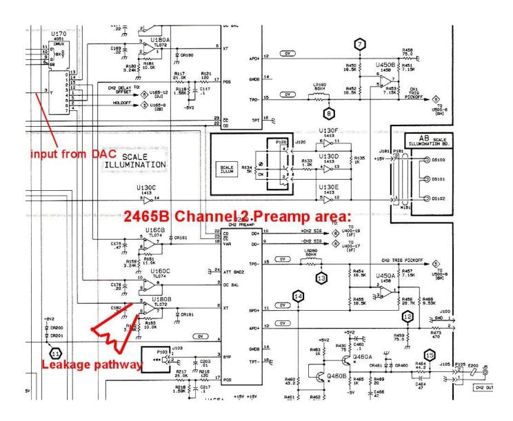
The effect of the leakage alters the DC input to the XT input of U200, the CH2 preamp IC. This resulted in a DC offset from U200's output. Surprisingly, further down the line this upset the operating conditions of U400 (the Channel Switch IC). This caused interactions of CH 2 with the other 3 channels and with the On Screen Data display.
