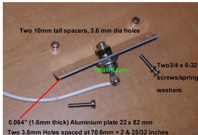
The photos below show the assembly screwed into the existing captive nuts:
