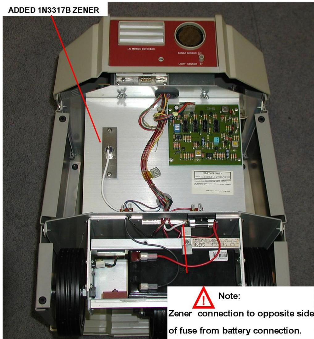
It is very important to connect the zener as shown above and **not** directly to the battery terminal. With over voltage or reverse polarity very high currents will flow via the zener diode and there must be a fuse in the circuit to prevent wiring burnup.
