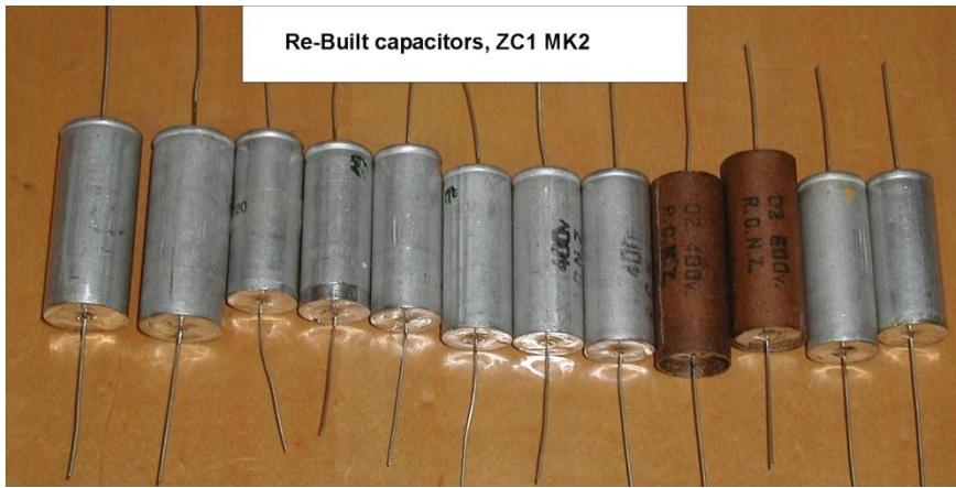
Two of the 0.02uF capacitors have external paper sleeves.
