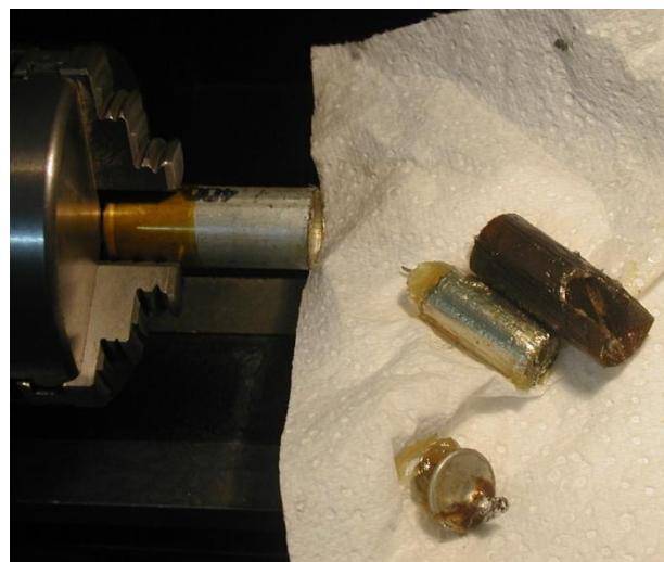
The photo below shows 5 of the cleaned out 0.1uF 400V capacitor canisters. Also the rivet and tag in the phenolic insulator is drilled out and discarded. I found these tags were in fairly poor order, the Brass being quite brittle where it was sharply folded and prone to cracking.
