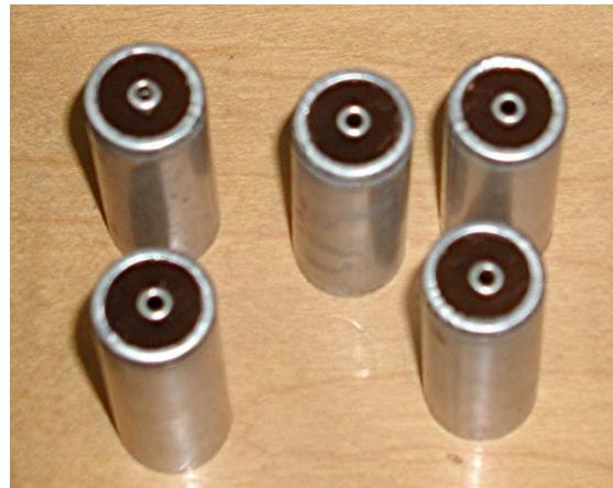
Then there is the issue of replacing the end of the capacitor which was cut off. A convenient choice is fibreglass pcb material. It is easily cut into discs using a 22mm diameter hole saw on the drill press. Then I make a 1/8" central hole and attach a screw & nut to secure it and rotate it, to machine the perimeter down to 16.8mm to be a close fit inside the end of the metal
