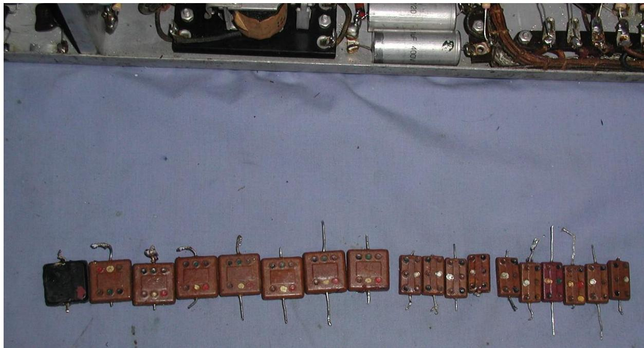
The photo below shows the underside of the ZC1 after re-capping. Of note nearly every carbon resistor except just a few in this radio, were way out of spec and I had replaced them in the past.
