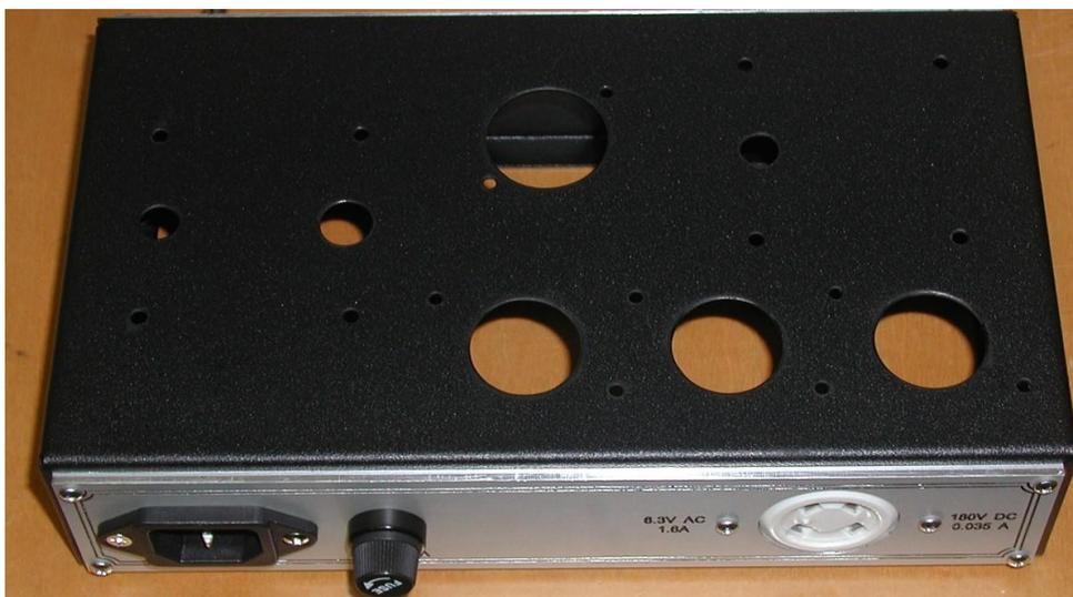
Also, I had the local engraving store make silver satin finish 3mm thick (close to 1/8") front and rear panels, engraving filled with gloss black paint. This shows the rear panel fitted.
