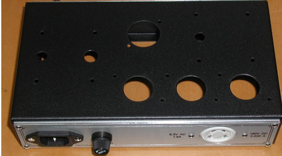
I have never been particularly happy with self threading screws into steel or aluminium sheet metal. I prefer pressed in nut inserts, so I abandoned Hammond's base screws and fitted 4-40 UNC stainless steel captive nuts for both the base plate & the top cover:
