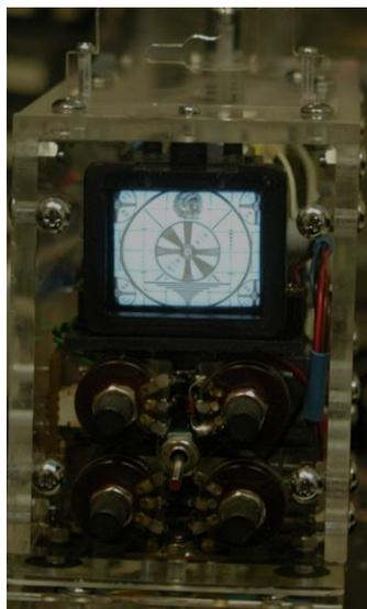
The acrylic panels for the case were hand sawn and smoothed on a flat surface with progressively finer grades of paper. Then with a cloth stretched on the surface and soaked in polishing compound the edges were polished by pushing the panels along this surface.
