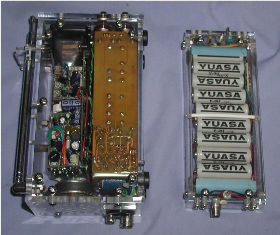
The above photo shows the battery pack unscrewed. The set itself is stand alone 230V mains powered, or battery and when the battery pack is attached, it trickle charges it. The battery screws were made from some old 1920 style knurled nuts from a valve socket:
