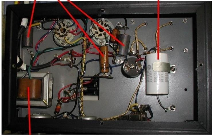
**Audio Opt transformer added to avoid high voltages rear panel connectors. 5.5k to 8 Ohm.**
