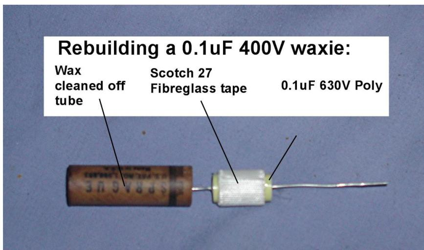
For the most part, doing large batches of waxies for TV restorations, I re-seal the ends by pouring them on alternate days with Polyester Resin. In this case for a one off I used 24 Hr Araldite. Also, I varnish the waxie with marine grade spar varnish (after the wax is removed, the varnish is miscible with the residual wax). This way they look good and the surface is non tacky and they don't stick to dust.
