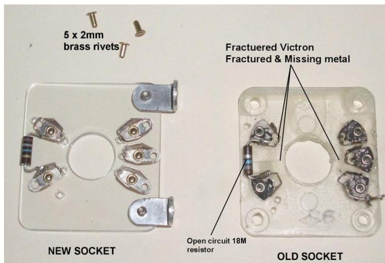
It was unexpected that the 18 Meg Ohm 955 tube's grid resistor was open circuit too. I replaced with a vintage 5% carbon composition resistor. It is important that this resistor does not have any inductive or reactive properties.
