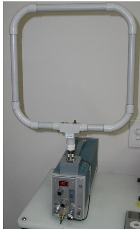
Fitting the F coil set to the 1-10 A I transmitted to it on 30.1MHz as an extended listening test. Once the regeneration control was set, it was perfectly stable. The audio output quality is excellent (especially with the broad range speaker attached, a vintage bookcase type) and the audio does not sound as bandwidth limited as it is on a standard Superhet radio. So it is a very pleasant listening experience.
