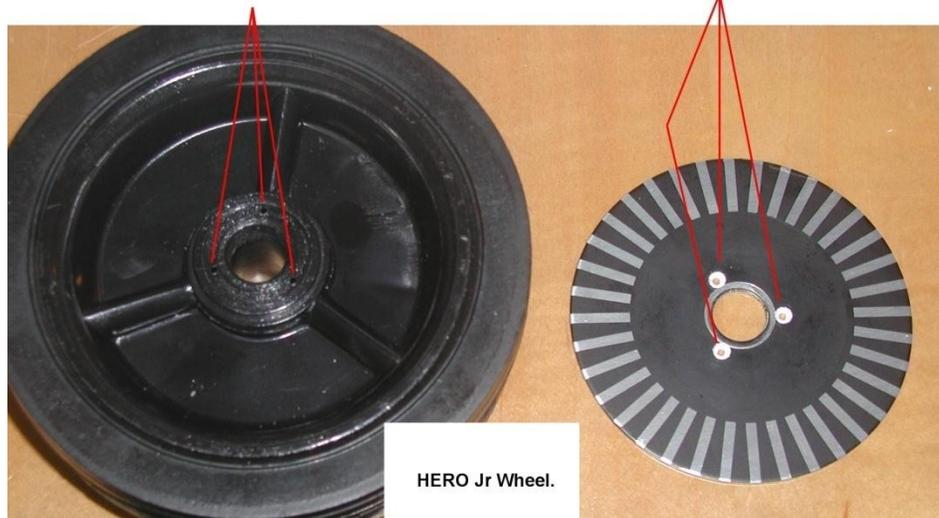
The 3 pilot holes in the wheel hub are then drilled to a depth of around 9mm with the 1.5 mm diameter drill. Once that is done a 2mm metric taper tap is used to start a thread into the initial part on the hole in the plastic hub, around 3mm deep. This allows the 2mm screw to start to screw in. Because the plastic is soft the 2mm screw makes its own thread as it is screwed into most of the 1.5mm diameter 9mm hole depth.
