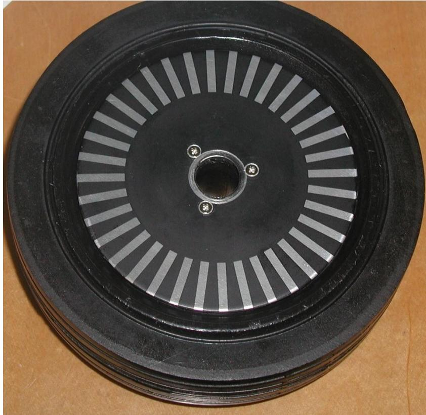
Although the nylon wheel hub itself has very low friction running on the aluminium bush, it does pay to apply some grease to make sure it runs as smoothly as possible.
