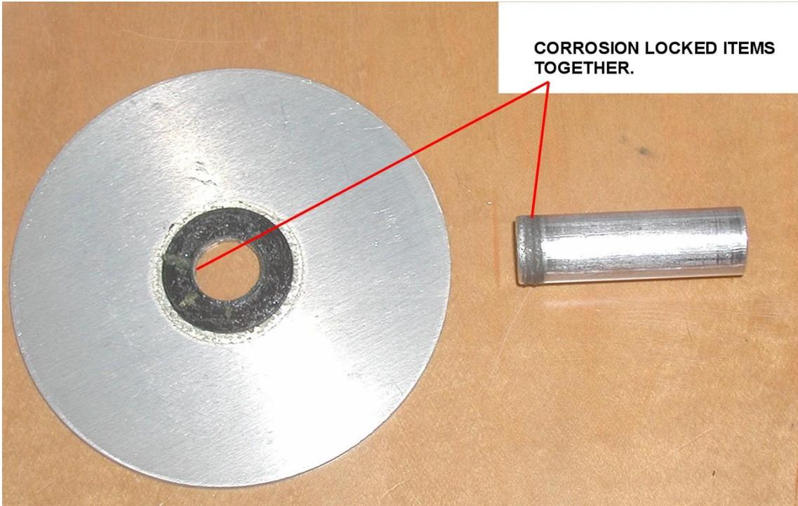
Inspection also revealed some other details. The wheel hub is made of particularly slippery plastic. I think it is most likely black Nylon. The glue used appeared to be a type of contact adhesive. While this worked reasonably well to glue the rubber spacer washer to the rear of the stroboscopic disc, it struggles to stick well to the wheel hub.
