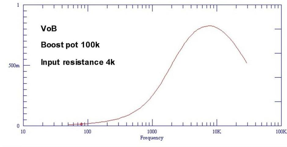
If everything is set to maximum, with the pickup controls at maximum and the boost level at maximum (minimum pot resistance) the following occurs. This up-shifted frequency response gives the Rally guitar an amazingly sharp cutting sound:
