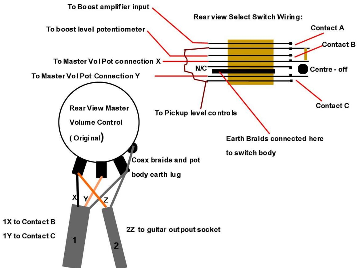
**Modified Master Volume Gretsch Rally: to allow Master Volume Control to operate in Treble Boost Mode.**
