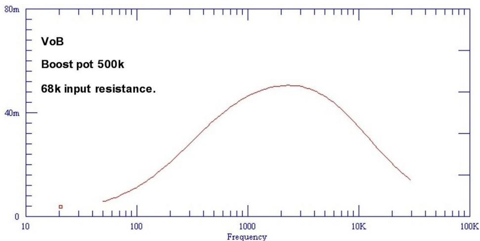
As can be seen from the above this setting of the maximum 500k for the boost control rolls off the very high frequencies and lowers the output level to a peak of only around 50mV or half the level of the input signal to the module, when that signal is sourced from around 68k, ie the pickup volume controls not quite at maximum. Also the frequency range of the response is down shifted.
