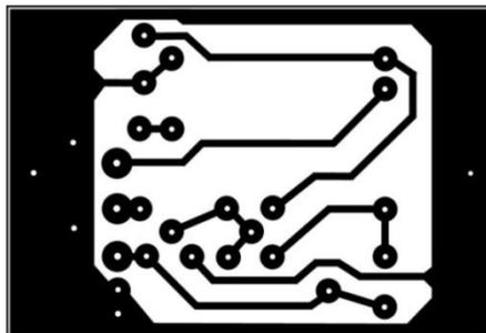
A replica pcb was made by printing the above images to iron on pcb film and then etching with ferric chloride. As noted small (1.6mm diameter) brass eyelets were fitted where the wires connect to make a stonger connection.
