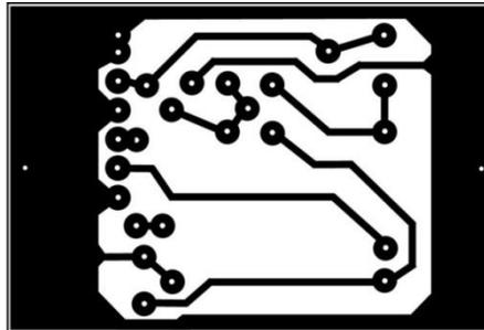
The image below shows the pcb as viewed from the top again and after a modification to space its connections a little wider apart. The original connections were a little crowded and spacing them a little allowed some small eyelets to be used on the replica pcb to make the wire connections a bit more solid and help protect the pcb track.
