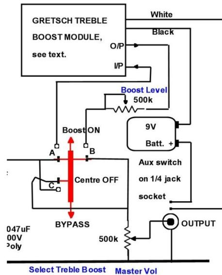
Which has the master volume control wired in a manner that one would expect. Another consequence of the original wiring is that a low volume setting, the resistance presented to the guitar amplifier's input is high, allowing more stray noise pickup. The way shown immediately above is better in this respect too.
