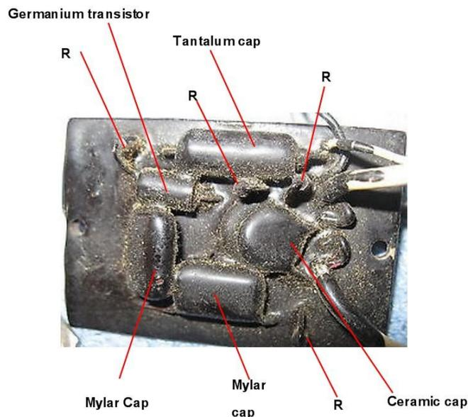
After this module was received it was found that there were in fact two ceramic capacitors, the other one can be seen through the black resin hiding under the one on top of it. Also the axial capacitor turned out to be an Italian made Ducati 15uF 15V, not a Tantalum, but Tantalum is better as it has lower leakage.
