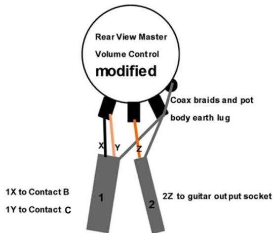
This results in the modified partial schematic:
