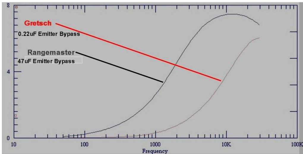
As can be seen due to the large value of emitter bypass capacitor (47uF) in the Rangemaster the frequency spectrum over which it boosts the signal is lower than the Gretsch module all other things equal. Since all of a guitar's fundamental notes lie in the
