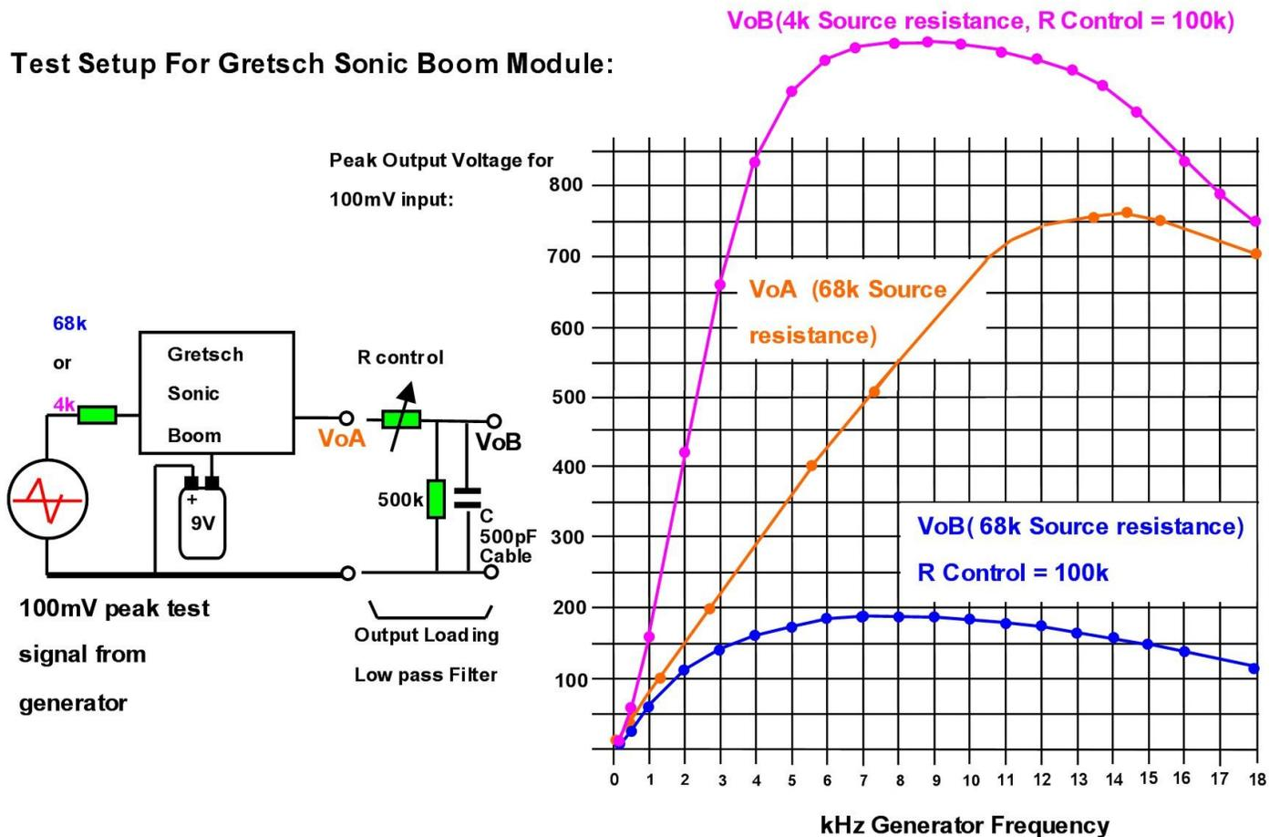
Under this test circumstance (orange graph) the boost unit acts like an attenuator for frequencies under 1000Hz and an amplifier with a gain of about +6 dB per octave with an input frequency above that. The attenuation is fairly heavy at around 100Hz. For example an open low E string is 82Hz.
