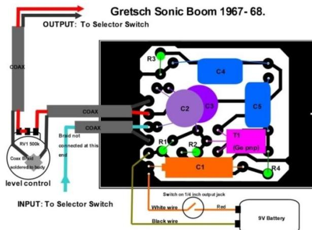
The pcb itself is 1.5 inch by 2.25 inch in size. The diagrams below also show the pcb track arrangement, bottom or track side view:
