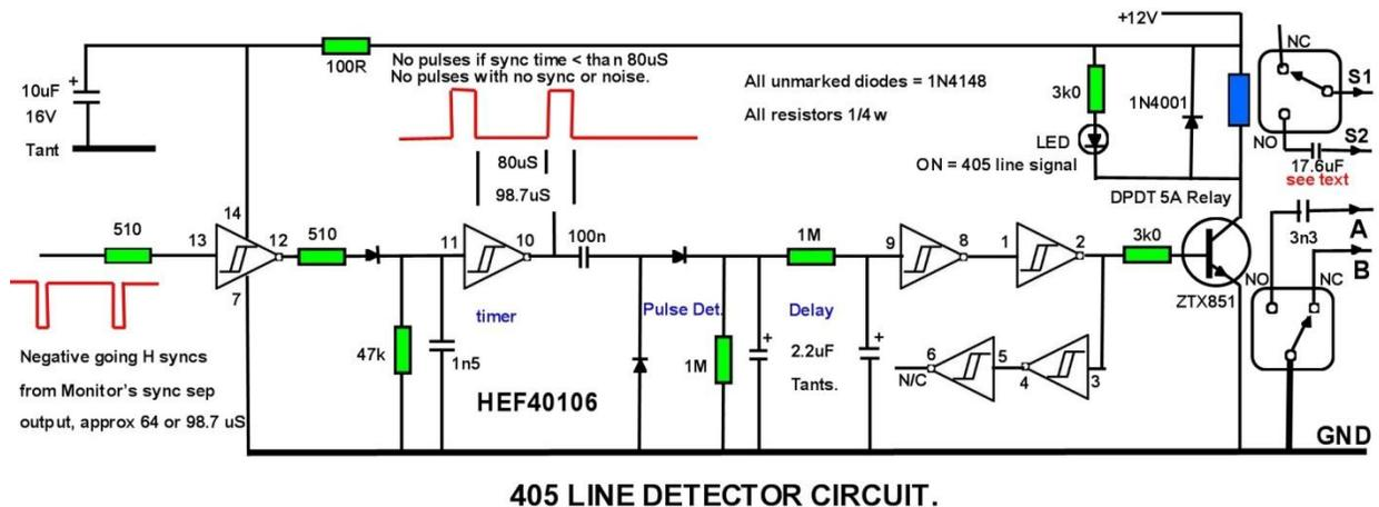
The monitor's separated horizontal sync pulse is inverted and used to charge a 1n5 capacitor, which fully charges during the width of the horizontal pulses. Between pulses the 1n5 discharges. If there is sufficient spacing between the pulses, in this case >80us then the threshold of the gate input (pin 11) is reached and the output of the gate (pin 10) goes high until the next sync pulse charges the 1n5 capacitor.
