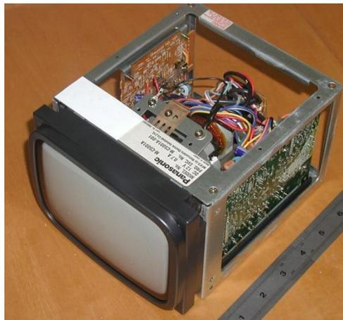
I had a few 5.5" diagonal industrial monitors, some of which I had already fitted with P4 CRT's. However, these monitors have no internal 12V power supply, so one would have to be added unless the monitor was run from a wall-wart supply which is a less favourable option. These monitors also have no front panel and no external controls and no outer case. All the controls are PCB presets.
