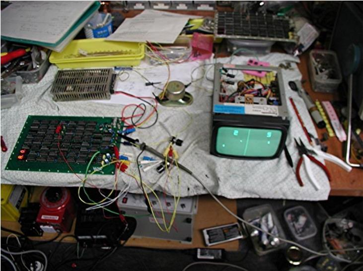
I find vintage series 74 TTL IC's very reliable. Perhaps one reason is that they are very robust to electrostatic discharge damage. Despite some remarks that back in the 1970's one in 100 or more might be faulty. In any event assembling the pcb above, from these new old stock parts which are over 35, some 43 years old, I powered the pcb and it worked perfectly first time. I think that says a lot about the quality and robust nature of the IC's.
