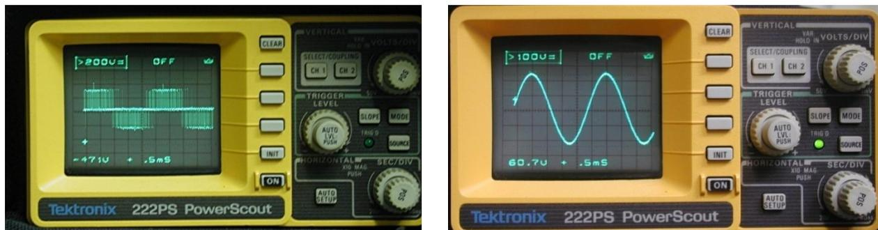
As shown in the photo, the sine wave filter does a very good job of re-assembling the PWM signal into a respectable sine wave. I was surprised how good filtered waveform looked, with the nature of the PWM signal, I was expecting more distortion. Under heavier loads than just the 3 lamps some small irregularities appear, but generally the waveforms are good.
