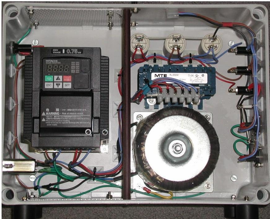
A large rectangular ventilation hole was cut above and below the inverter and fitted with a perforated aluminium panel. The entire case is on large rubber feet so there is a good convection current through the unit and past the VFD's heat sink. The VFD is rated to 750W, so this unit can easily supply two 60 watt monitors at once and it only gets a little warm, most of the heat being from the indicator lamp/loads, not the VFD itself.
